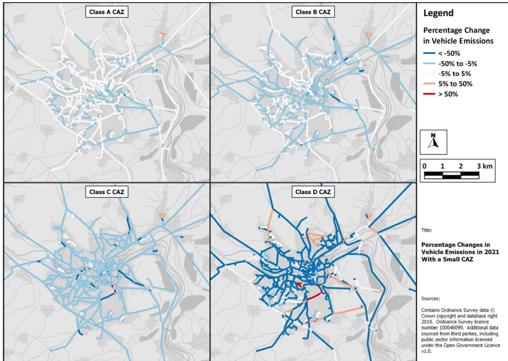
Figure A.1 - Percentage Changes in Vehicle Emissions in 2021 With a Small CAZ
